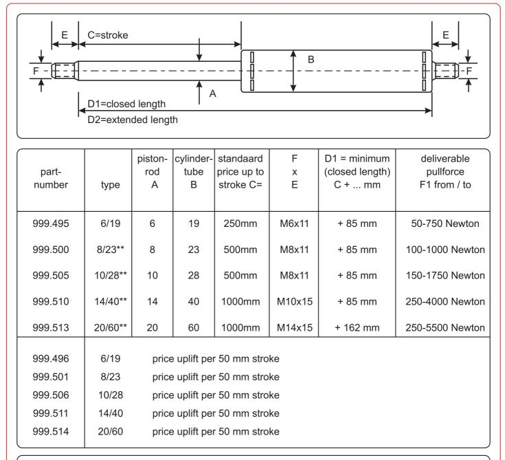
The piston rod is hard chronium plated and the cylindertube is zink plated.
