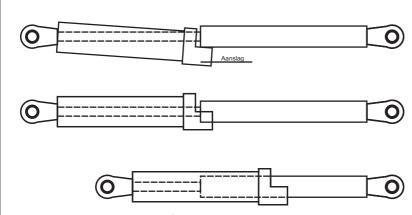
These safety / protection tubes offer protection against unintentional closing of hatches / covers and pro-. tects the piston rods from damaging. Are complete stainless and therefor Usable with stainless steel gas push and pull springs.
